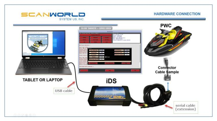
After you connected computer – iDS – vessel/vehicle you can start your software
